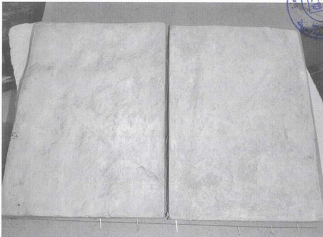
Fig 2 the artificial stone before and after weathering exposure
